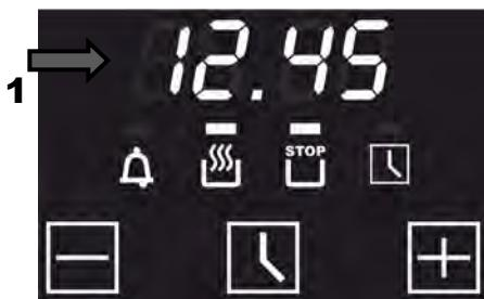
The end time **1** appears on the display, that accords to the current day time plus duration (in our example **12:45**, that means plus 30 minutes).
