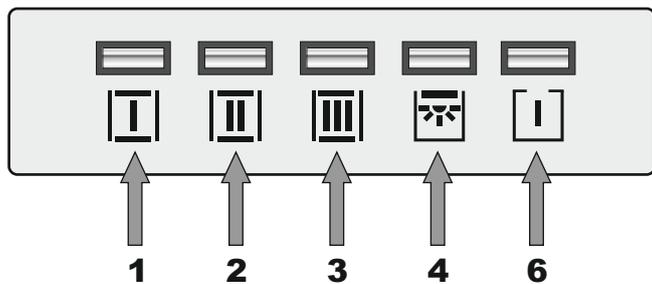
According European Norms 65/2014 and 66/2014 the hood with motor power more that 260W may work on high speed **3** only 7 minutes, after 7 minutes the speed is changed to medium speed **2** automatically.
